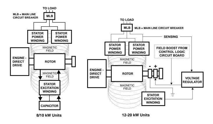
Figure 1. Operating Diagram of AC Generator
